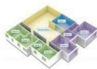
Being air-con experts, we couldn't leave it there. We've also dumped the wasteful dump zone. In standard systems, this large zone can occupy up to 25% of your home. It is permanently open to stop air pressure build up blowing your ductwork out of place. With the Zone 10, an electronic default constant monitors the system and only opens a pre-selected dump zone when needed.
